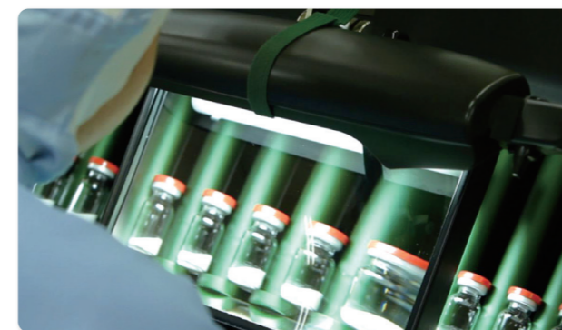
Visual inspection of lyophilized products to detect foreign particles.
